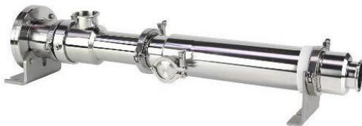
The progressive cavity pump is particularly suitable for conveying and filling abrasive and solid-containing media. The abrasive solids are transferred in a product- and pump-gently way in the carrier medium through the chambers between the rotor (stainless steel) and stator (elastomer). The friction coefficient between rotor/stator combinations is reduced through the tribological film of a few  $\mu\text{m}$ . Therefore premature wear is avoided.
