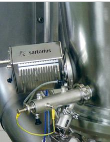
NIR spectroscopy and imaging with the PMD500 for use in the powdered milk production process.
