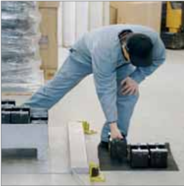
Figure 4 During installation, a scale should be adjusted to the ambient conditions as needed.
