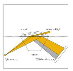
If a CCD line is used for detection, the temperature must be precisely measured in order to maintain the accuracy of the refractometer.
