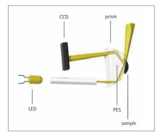
They do not have any moving parts, making them very robust and resistant to defects. To a great extent, the quality of the central components determines the measurement accuracy and reliability of a refractometer
