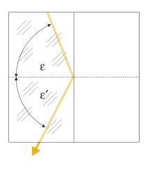
When light travels from one medium to another, part of the light is refracted, and the other part is reflected depending on the refractive index difference and angle of incidence. With unpolarized light, the proportion of reflected light constantly increases with the angle of incidence up to the critical angle of total reflection. This relationship is shown in the following figure:
