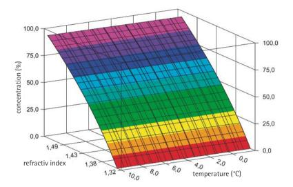
To create a scale, this surface must be adapted using a polynomial. The quality of this polynomial determines the measurement accuracy of the refractometer. A high refractive index resolution is useless if the polynomial is of low quality. To achieve a high degree of measurement accuracy and reliability, it is absolutely essential that the developed user-defined scales are very complex and sophisticated.
