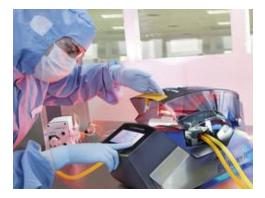
The thermal weld produced by BioWelder® TC ensures an extraordinary level of stability, thus guaranteeing an ultra-safe connection. The thermal weld has been qualified by applying the most stringent and innovative test regimes. Biological, physical and extractables tests were combined to obtain data representing a variety of process conditions, including critical applications.
