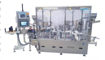
Transport within the machine is done extremely gently without any glass to glass contact. Assembly functions for additional components and camera systems can be integrated as an option. The machine that flexibly handles a variety of formats achieves a capacity of up to 3,200 syringes an hour.
