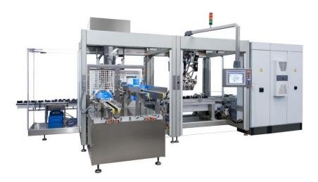
Optima Consumer is displaying the new high-performance OPTIMA CBF cartoner. This bridges the gap between primary and secondary packaging for perfect line integration. The products fed to the machine are aligned and placed within the cartoner. The flexible structure also makes a most convincing impression. Product grouping devices or a second
