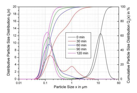
Illustration 1: Development of the particle size distribution obtained during a grinding test in a laboratory bead
