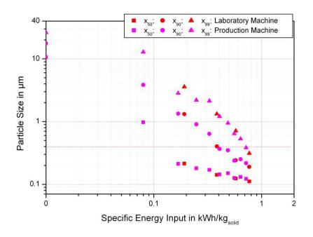
Illustration 2: Results of the scale-up from a laboratory agitator bead mill to a production-size mill
