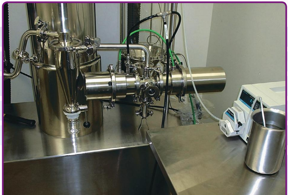
Figure 3: In-line particle size analyzer installed on the existing line from a GEA Spray Dryer type SDMicro™
