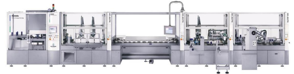
Dividella's machines are modular in construction and individually tailored to customers' requirements; if these requirements change over time, the modular construction of Dividella machines means they can be upgraded to meet the new requirements perfectly.
