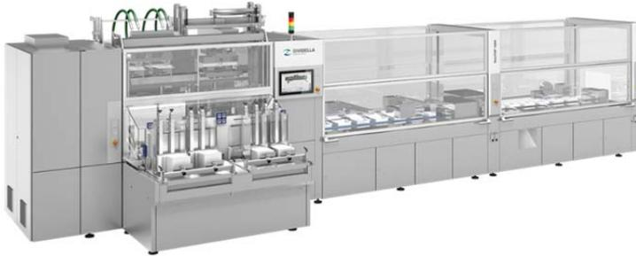
*The NeoTOP 1604 is ideally suited for packaging medium-sized and large lots up to 16 million packs per year. With its large format range blisters, ampules, vials, syringes, injectors and similar products can be packaged in a wide range of standard and special packs.*
